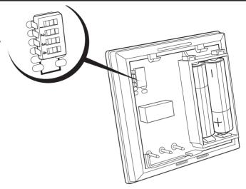
**ON/OFF** - boiler switches ON when below set temperature and OFF when above.
