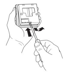
Fix at a height of 1.5m approx from the floor, away from draughts or heat sources such as radiators, open fires or direct sunlight.
