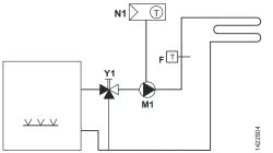
Room thermostat for control of electric floor heating systems. Floor temperature limitation with cable temperature sensor Room thermostat with direct control of hydronic floor heating system
