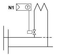
Room thermostat for a hydronic radiator or floor heating system
