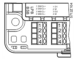
LPB/BSB Digital D1 DB/CL+ 1 DB/CL+ 2 М 2 MB/CL-D2 3 3 MB/CL-Μ 4
