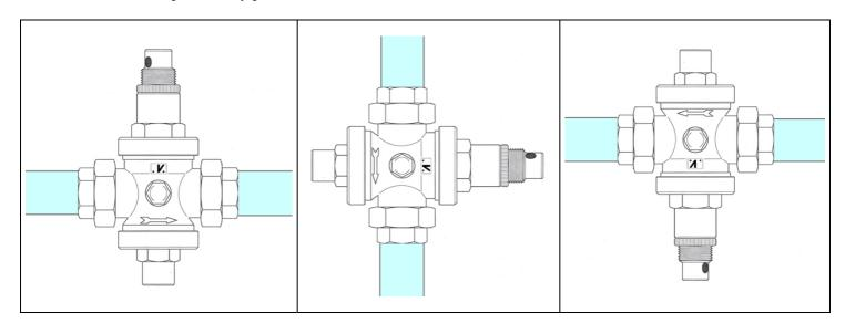
Pressure reducing valves can be damaged by dirty water; therefore we advise to install a self-cleaning filter upstream before the pressure reducer, in order to protect the valve and any other mechanism.
